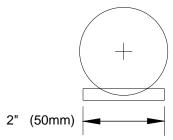
Pinheads with a flat anchor larger than 2 1/2" (63 mm) can be trimmed and ground. \*NOTE\* a flat portion must be retained to stop pin from turning during assembly. Key stock stop maximum 2" (50 mm) long allowing core to be welded into position.
