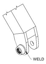
Assemble snubber with slot style housing facing down parallel to link. An anchor must be cut from 1" (NORTH AMERICA) 25 mm (EUROPE) steel plate and welded to link. Maintain 1/8" (3 mm) clearance between bottom of housing slot and top of anchor, allowing full engagement of anchor.
